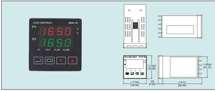
The compact Series 16C Temperature Controller offers accurate temperature measurement and control in a 1/16 DIN package. Designed for direct or reverse acting (cooling or heating) control, the Series 16C can be programmed for simple ON/OFF or more complex PID control functions. PID control is supported with manual or autotuning. Select relay, voltage or current output for control methods.
