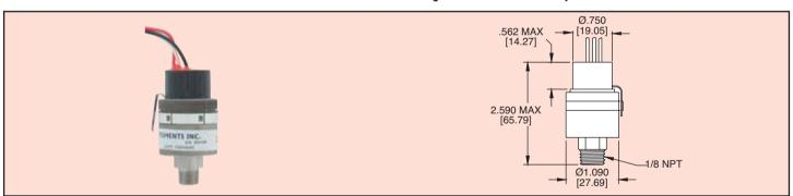
Miniature Series APS/AVS Adjustable Switches offer reliable switching for pressure/vacuum alarm, shutdown or control. The units are readily adjustable throughout their range using the locking adjusting ring and indicating pointer. The body is constructed of stainless steel for durability in harsh environments. Switches include 12" (30 cm) wire leads sealed with epoxy for additional protection.
