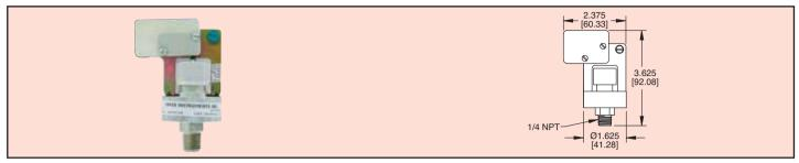
Series A1PS/A1VS Economical Pressure Switches are designed with a 15 Amp SPDT switch for direct control of pumps and motors. Available in pressure, vacuum, or compound ranges, the switches offer a field adjustable set point. Easily adjust the switch by aligning the top of the self locking adjusting nut with the desired setting indicated on the adjacent range scale. Connection is 1/4" male NPT for quick installation and can be mounted in any position.
