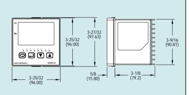
The Series 4B 1/4 DIN Temperature/Process Controller is designed to accept thermocouple, RTD, current or voltage input and provide dual outputs for control. Available outputs include relay/relay, voltage pulse/relay, current/relay, or linear voltage/relay.
