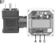
To program, first remove the cover from the indicator housing and identify the buttons A, B, and C. These buttons are used to program the indicator to match the pressure range of the transmitter.
