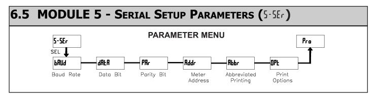
The Serial Setup Parameters are only active when the optional RS232 or RS485 serial communications module is installed in the meter.
