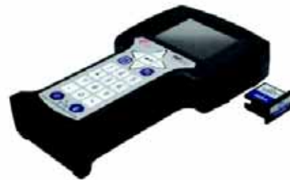
FIGURE 5. The Configuration Expansion Module safely stores hundreds of device configurations.
