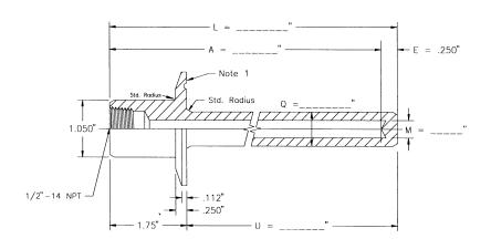
Note 1: Manufactured one piece construction with dimensions to mate to industry standard end caps.
