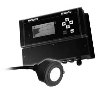
The MSL600 sludge blanket monitor is a microprocessor based system, with an abundant range of built-in display, control and alarm features. Easy to use menu driven programming allows complete configuration of the unit in just a few minutes. Local programming is carried out via an on-board membrane keypad.
