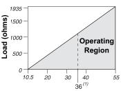
Power Supply Output Code S (dc Volts)
